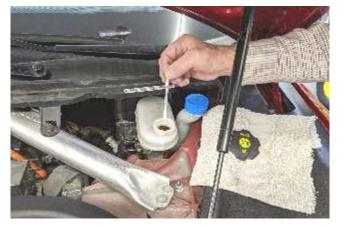
The right photo shows a test strip being immersed into the master cylinder of a Tesla. We measured two cars and the Miata showed "0" contamination and the Tesla strip showed about 10 ppm. Both were much less than the 200 ppm threshold for replacement. Will recheck annually.
